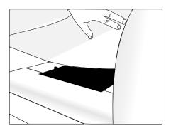
When installing the pad make sure the cable can't cause a trip hazard.
